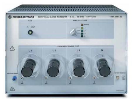
The Four-Line V Network R&S ENV 4200 is used for measuring RFI voltages on AC supply connections of EUTs carrying very high currents. It uses air-core inductances and contains an artificial hand. The R&S ENV 4200 satisfies the requirements of CISPR 16-1, VDE 0876 and ANSI C 63.4 for V networks with an impedance of 50  $\mu$ H  $\parallel$  50  $\Omega$  in the frequency range 150 kHz to 30 MHz.
